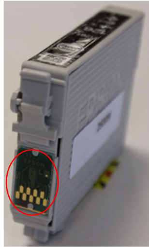
Genuine Epson Group 1 Cartridge (Control # 250086) With printed circuit board with terminals circled in red
