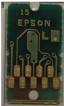
Enlarged view of printed circuit board showing the cartridge's terminals
