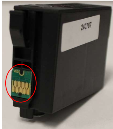
Group 1 Accused Ink Cartridge Product (Control # 240787) from Proposed Respondent Mountain Peak with printed circuit board with terminals circled in red
